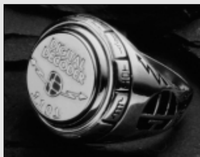
Photo 1. Decoder rings such as this one incorporating an iButton can serve as a convenient replacement for employee identification badges. The button can contain up to 64 K of memory to record security level, personnel or medical data, etc.
